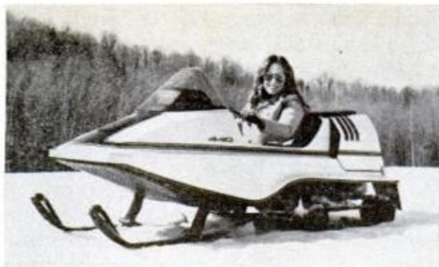
FRESH THINKING in snowmobile design is seen in Leisure Vehicles' Raider. Driver steers from cockpit seated over twin-track system; no leaning necessary
